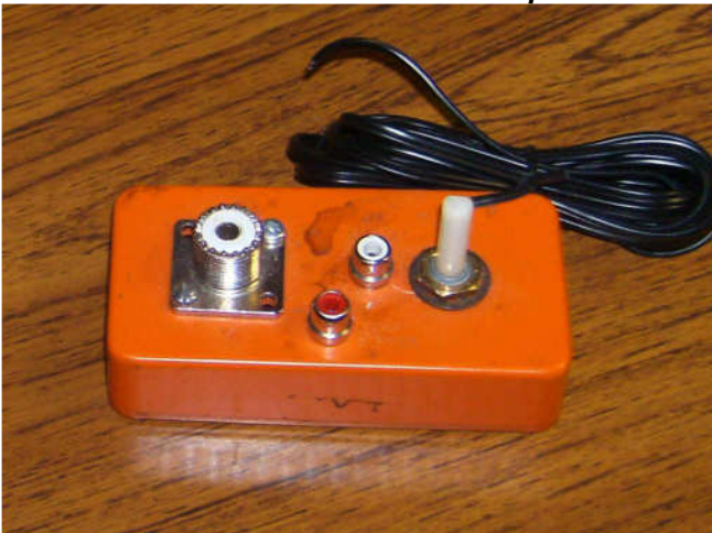
G6DTW VCR adapter for recording MF/HF spectrum
