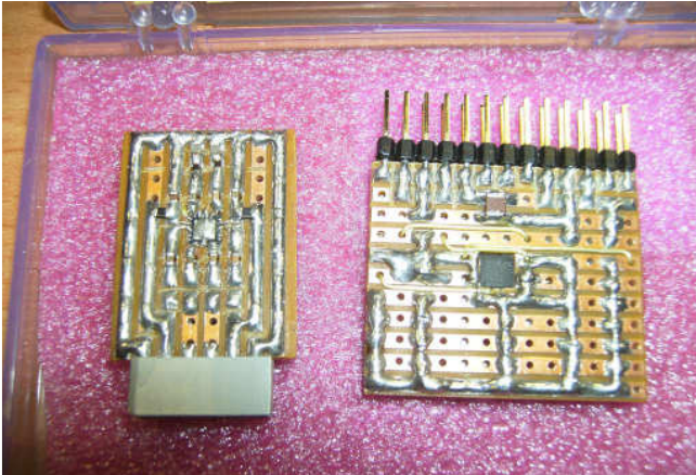
G3OQD Mini Veroboard based PCBs for surface mount components for SDR
