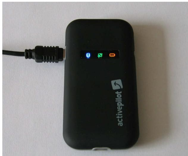
The device is intended to be used with mobile phones and PDA's that have a mapping application capability but no GPS receiver.
