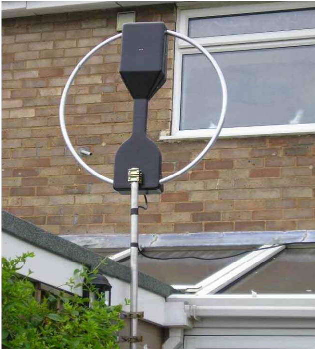
G7ELG's MFJ Magnetic Loop 10-30MHz
