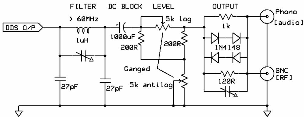
I had to hand a 5k log/antilog pot that I included as an adjustable attenuator whilst maintaining a reasonably constant output resistance to the filter. A phono connector was added for application at audio frequencies. It has been noted that the DDS output falls steadily above about 30MHz. The R/C combination in series with the RF output BNC flattens this effect to some extent (trimmers are 20pF).
