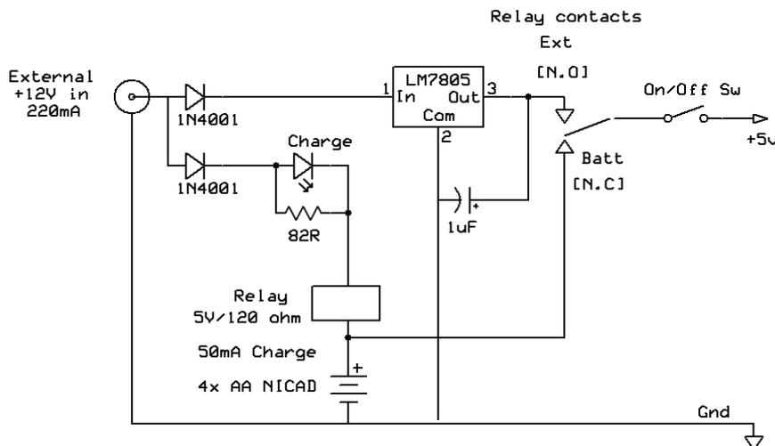
With no external supply, DDS is powered by wired-in nicads. Applying external 12V energises the relay and 5V is delivered via the voltage regulator. At the same time, current then flows through the LED and relay coil resulting 150mA or so to charge the nicads.
